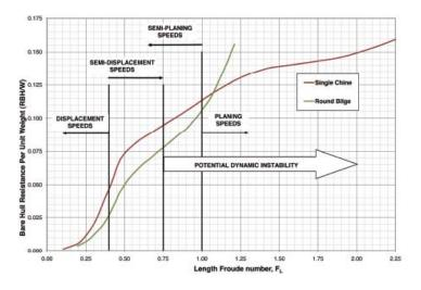
length, speed, and wetted surface area of the hull. Wave-making characteristics are related to two non-dimensional similarity parameters, one called Froude Number that is a function of speed (V) and waterline length (L) and another parameter related to the pressure forces acting upon the hull bottom. When Froude number is calculated based upon length, it is called the Length Froude number, FL=V(gL)1/2, where g is the acceleration of gravity.
