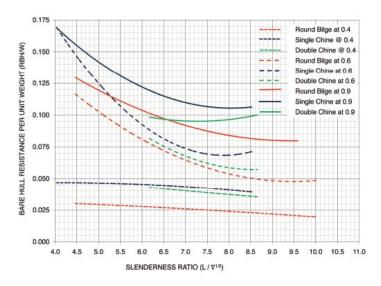
For semi-planing yachts, similar trends for single chine and round bilge yachts can be observed but the rate of bare hull-resistance reduction as slenderness ratio increases is lessened. Interestingly, the limited amount of available data for double chine hull suggests that the influence of slenderness ratio is quite muted and at a slenderness ratio of around 6.0 to 6.5, a double-chine hull form may offer the least resistance.
